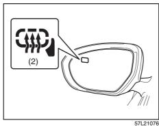
If the outside rearview mirror has the mark (2), it is also equipped with the heated outside rearview mirrors. When you push the switch (1), both the heated outside rearview mirrors and the heated rear window will operate simultaneously.
